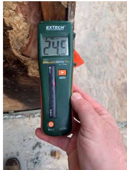
Photograph 4 Moisture content reading at the northeast corner.
